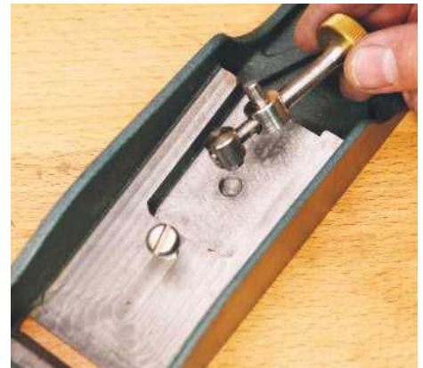
▲ A large milled bedding surface on the low-angle jack gives great support
